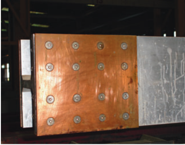
Terminal of the bar: a copper plate is positioned at the end of the bar for perfect current conductivity.
